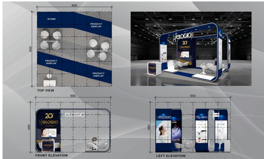
C.2 (1)- Example of Orthographic View- Top, Side , Front and Back grid/elevation drawing with measurements
